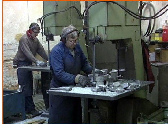
FIG. 45 - WORK WITH THE BELT SAW
