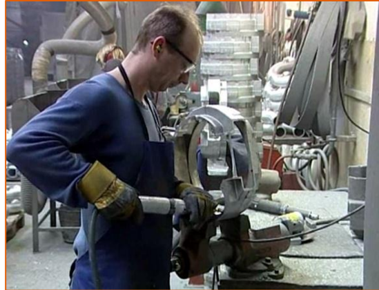
FIG. 47 - WORK WITH THE MANUAL GRINDER
