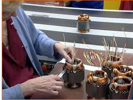
FIG. 51 - FINAL ASSEMBLING OF WINDING
